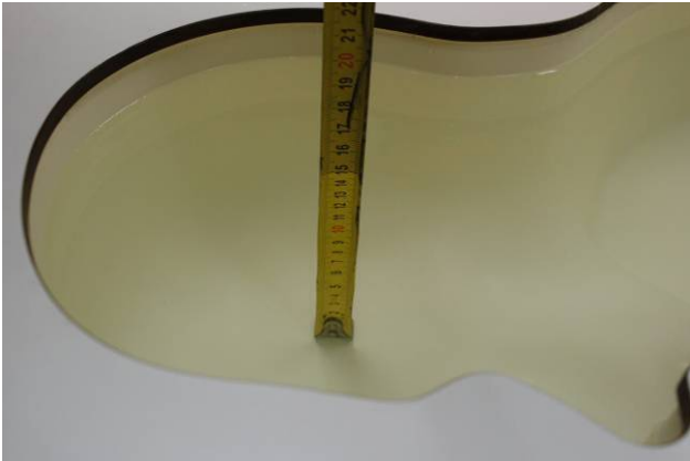
Liquid depth in the head Phantom (1800 MHz 15cm depth)
