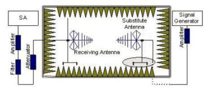
In the chamber, an substitution antenna for the frequency band of interest is placed at thereference point of the chamber. An RF Signal source for the frequency band of interest isconnected to the substitution antenna with a cable that has been constructed to not interfere with
