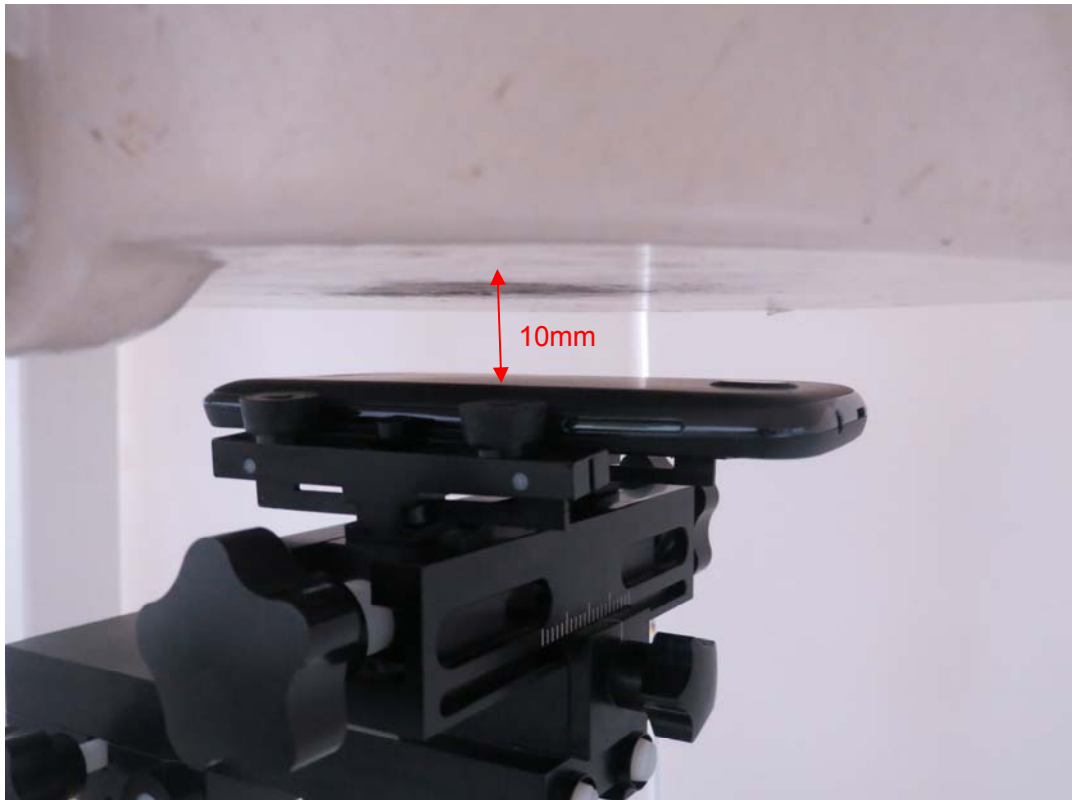
Picture 9: Back Side, the distance from handset to the bottom of the Phantom is 10mm
