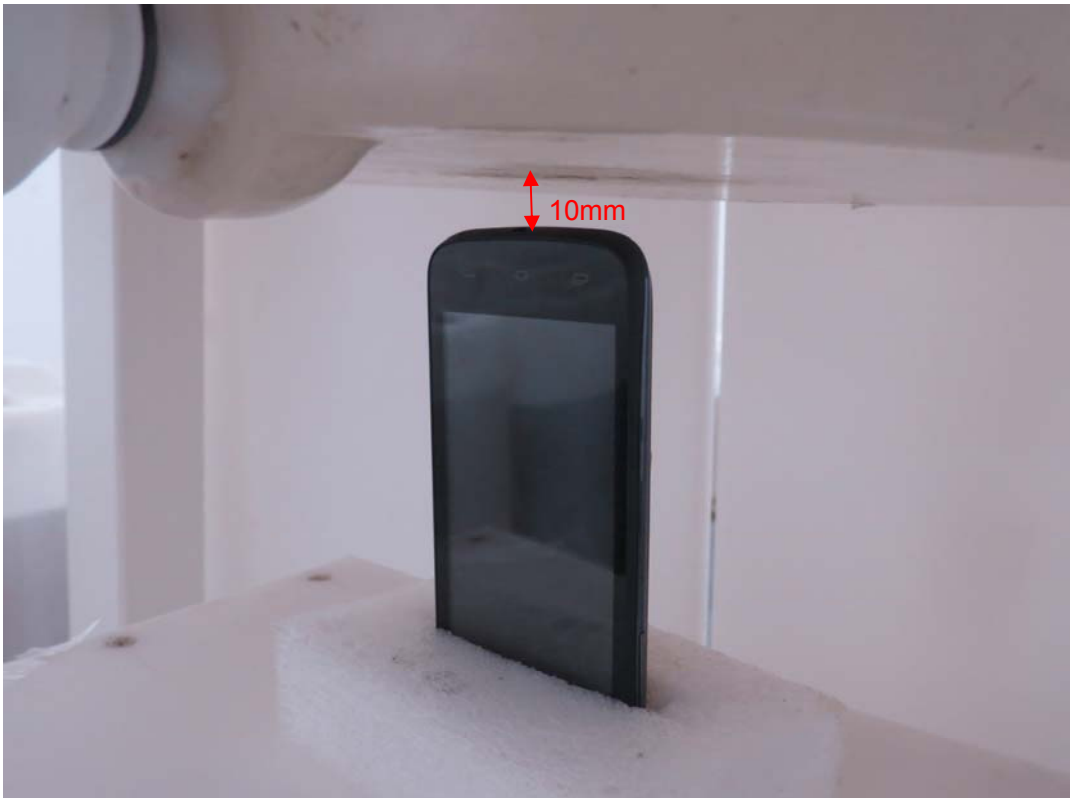
Picture 14: Bottom Edge, the distance from handset to the bottom of the Phantom is 10mm
