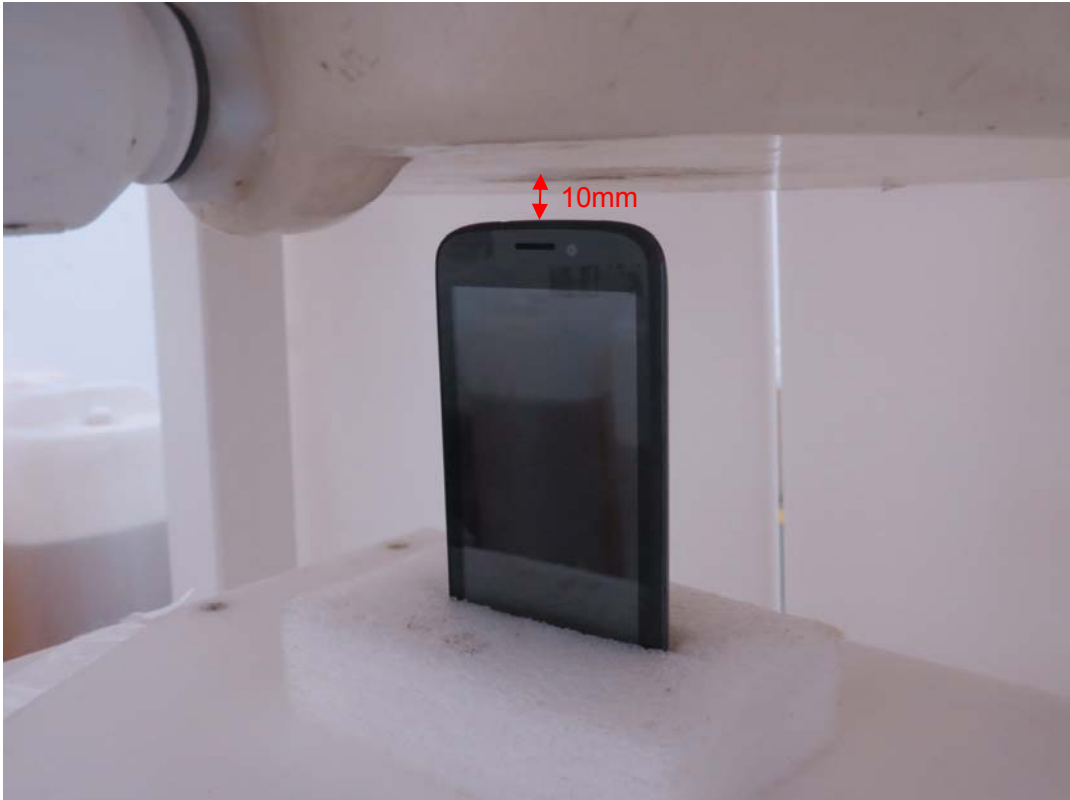
Picture 13: Top Edge, the distance from handset to the bottom of the Phantom is 10mm (This position does not need to be tested)
