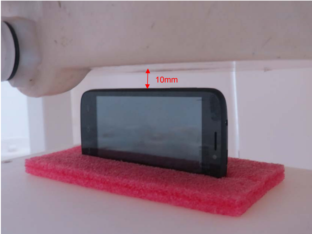
Picture 11: Left Edge, the distance from handset to the bottom of the Phantom is 10mm
