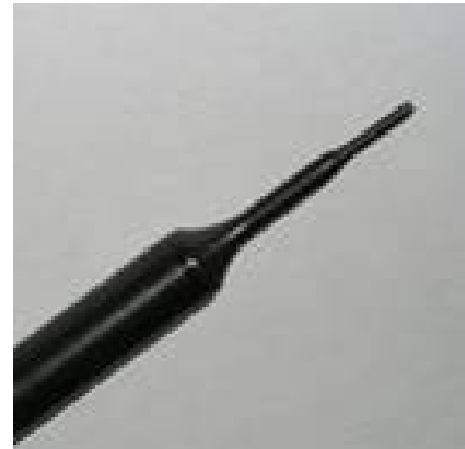
Figure 2. EX3DV4 E-field Probe
