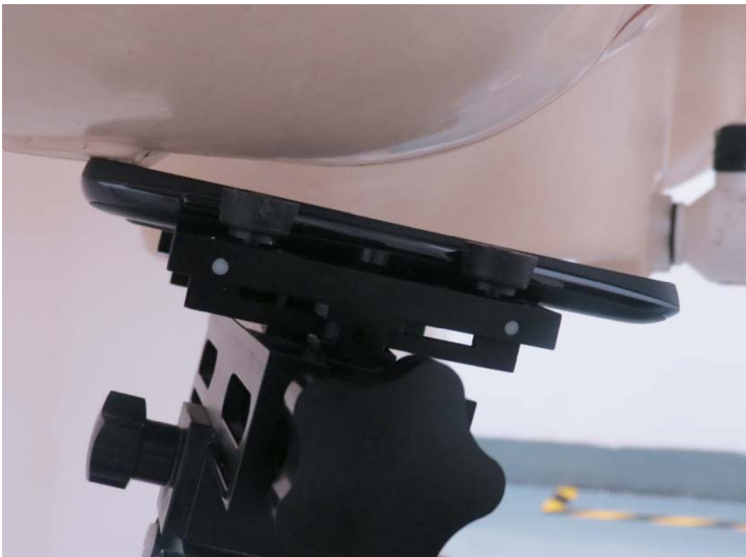
Picture 8: Right Hand Tilt 15 Degree Position
