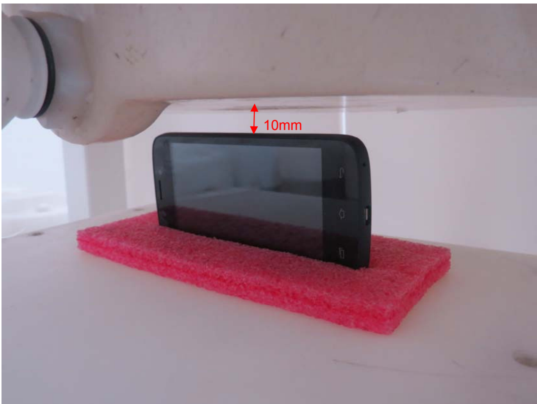
Picture 12: Right Edge, the distance from handset to the bottom of the Phantom is 10mm (This position does not need to be tested)
