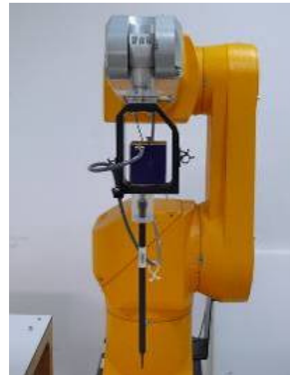
Figure 3. EX3DV4 E-field probe
