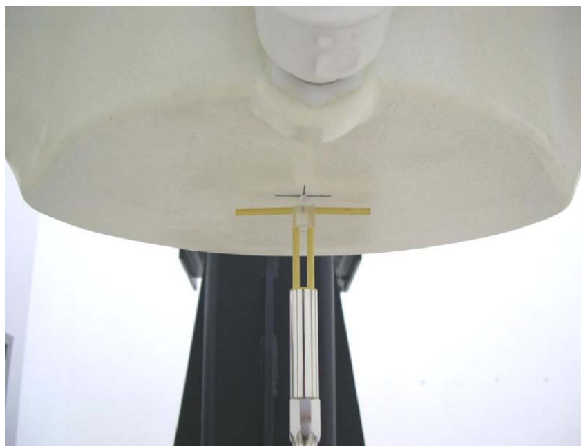
Picture 8.2 Photo of Dipole Setup
