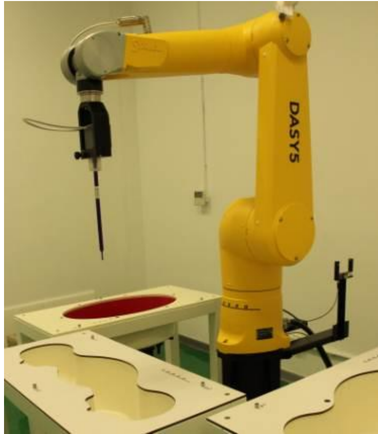
Picture D.6 DSY5 system Set-up
