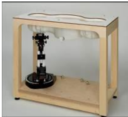
Picture C.9: SAM Twin Phantom
