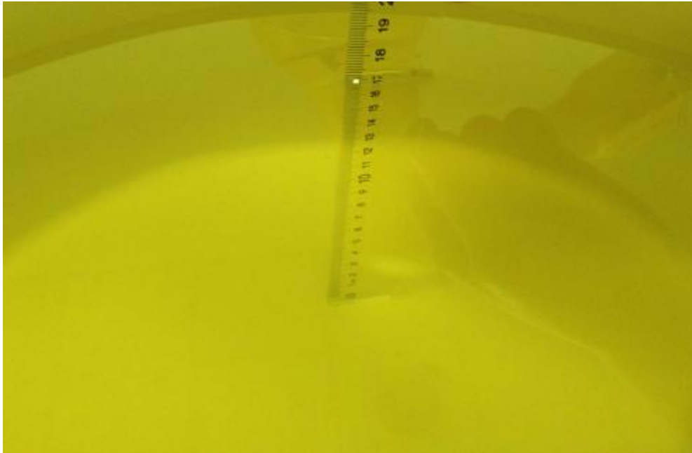
Picture 7-2: Liquid depth in the Flat Phantom (1900 MHz Head)
