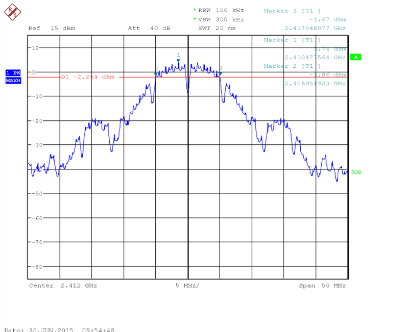
Fig.13 Occupied 6dB Bandwidth (802.11b, Ch1)
