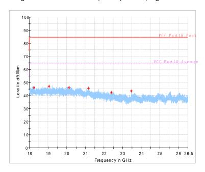
Fig.45 Radiated emission: GFSK, 18 GHz - 26 GHz
