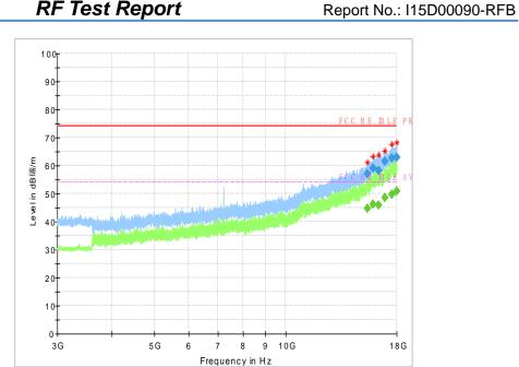
Fig.42 Radiated emission: GFSK, Ch0, 3GHz~18GHz
