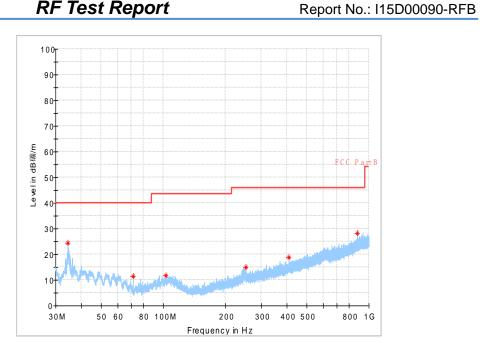
Fig.52 Radiated emission: 8DPSK, Ch0, 30MHz~1GHz
