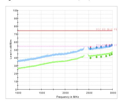
Fig.47 Radiated emission: π/4 DQPSK, Ch0, 1GHz~3GHz
