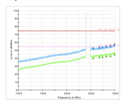
Fig.41 Radiated emission: GFSK, Ch0, 1GHz~3GHz
