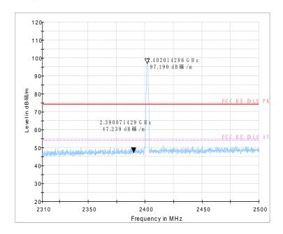
Fig.55 Radiated emission (Power): 8DPSK, low channel
