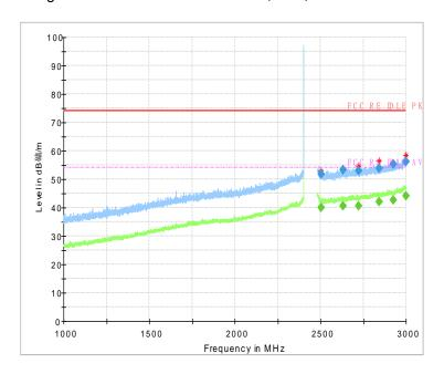
Fig.53 Radiated emission: 8DPSK, Ch0, 1GHz~3GHz
