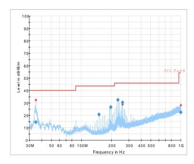
Fig.40 Radiated emission: GFSK, Ch0, 30MHz~1GHz
