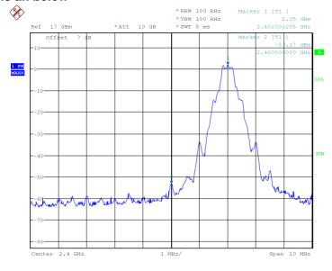
Fig.10 Frequency Band Edge: GFSK, Ch0, Hopping OFF
