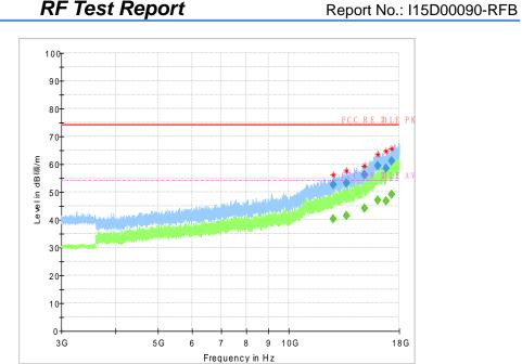
Fig.54 Radiated emission: 8DPSK, Ch0, 3GHz~18GHz
