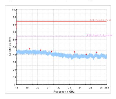
Fig.57 Radiated emission: 8DPSK, 18 GHz - 26 GHz
