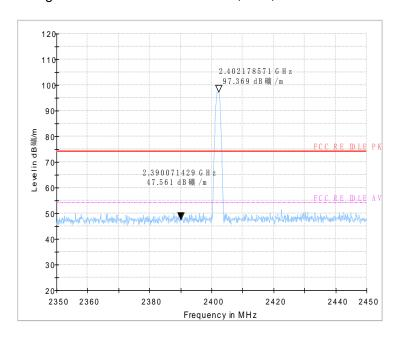
Fig.43 Radiated emission (Power): GFSK, low channel (peak)
