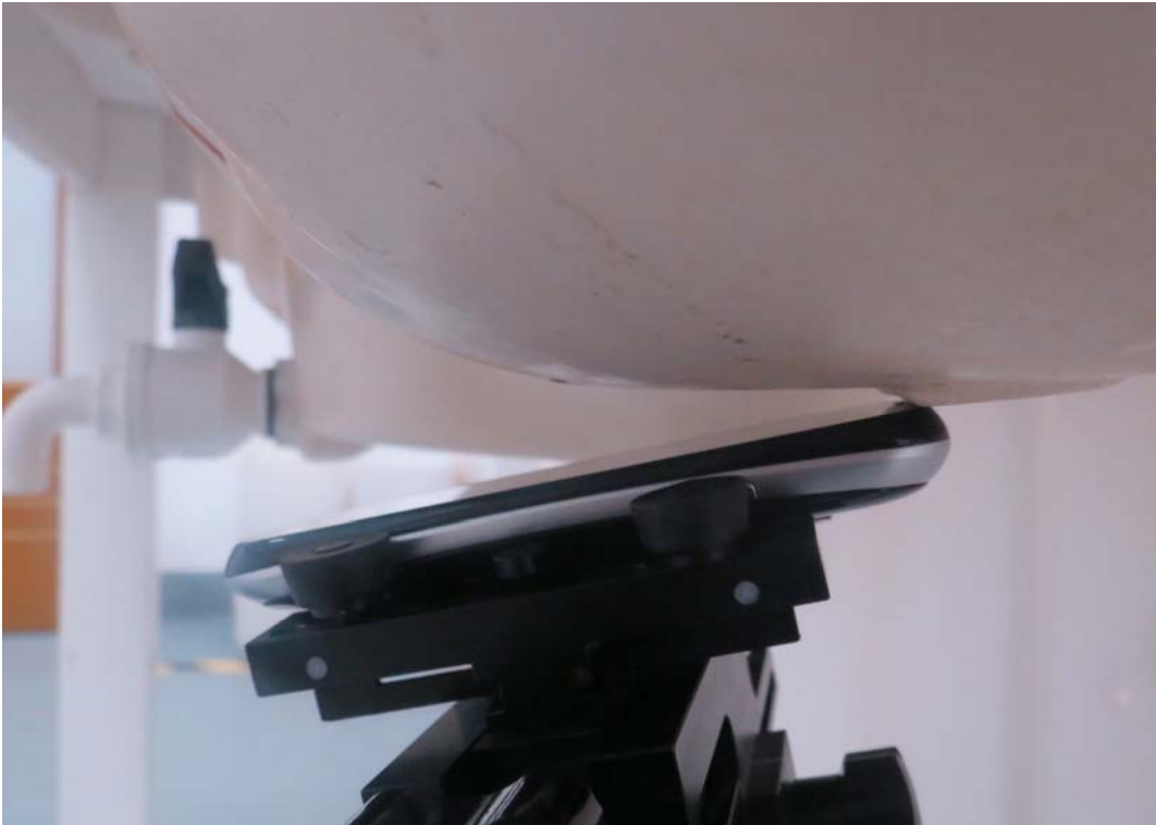
Picture 6: Left Hand Tilt 15 Degree Position(Original)
