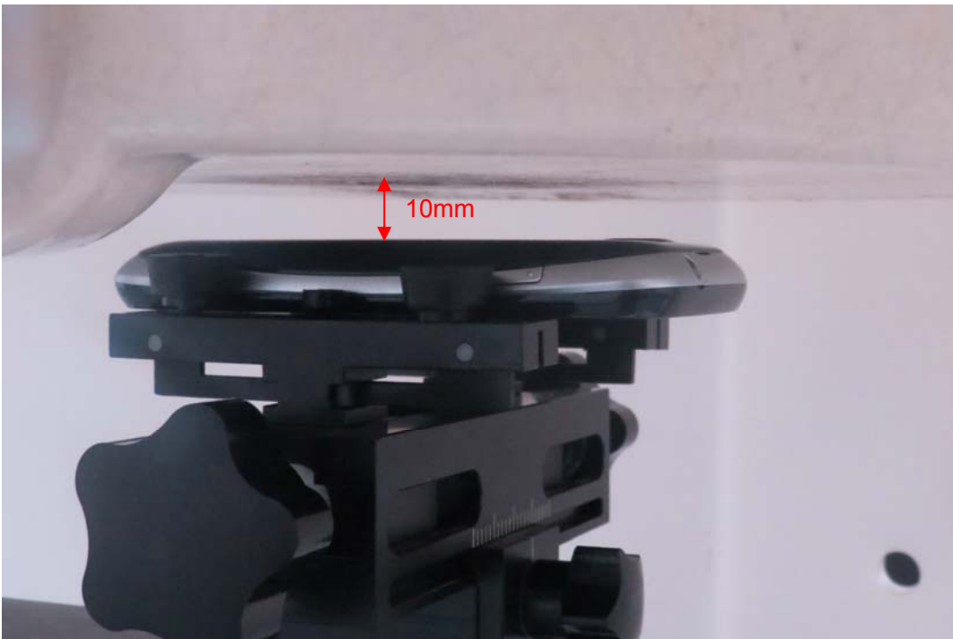
Picture 9: Back Side, the distance from handset to the bottom of the Phantom is 10mm(Original)
