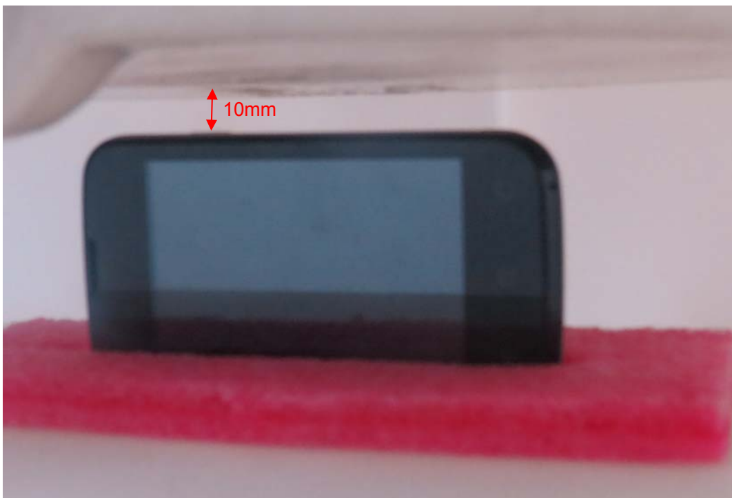
Picture 12: Right Edge, the distance from handset to the bottom of the Phantom is 10mm(Original)
