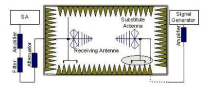
In the chamber, an substitution antenna for the frequency band of interest is placed at thereference point of the chamber. An RF Signal source for the frequency band of interest isconnected to the substitution antenna with a cable that has been constructed to not
