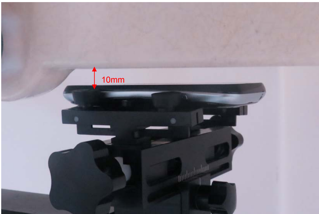
Picture 10: Front Side, the distance from handset to the bottom of the Phantom is 10mm
