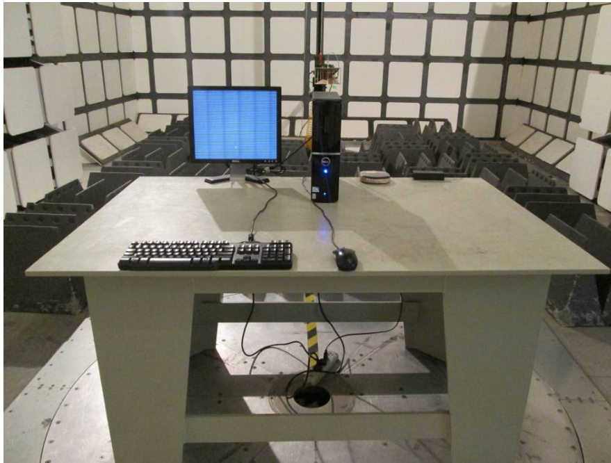
Radiated Emissions - Front View (Above 1 GHz)
