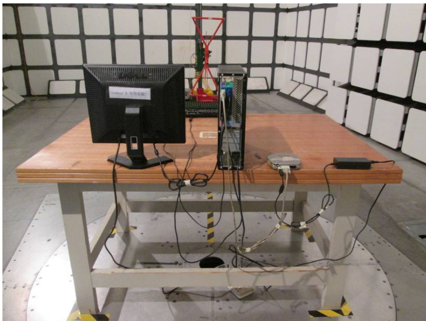
Radiated Emissions - Rear View (Below 1 GHz)
