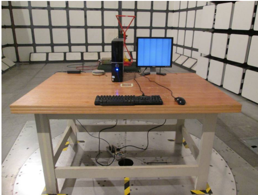
Radiated Emissions - Front View (Below 1 GHz)
