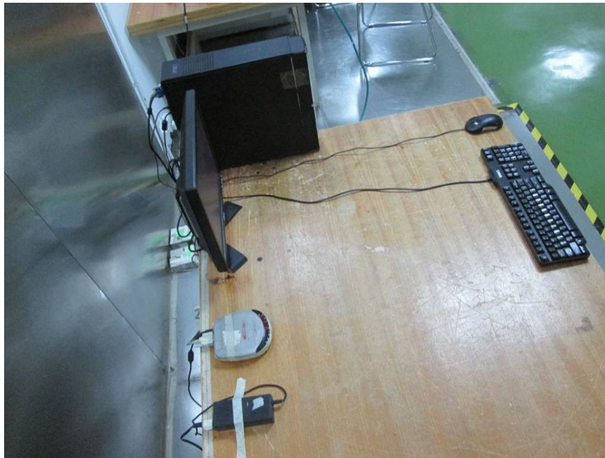
Conduction Emissions – Side View
