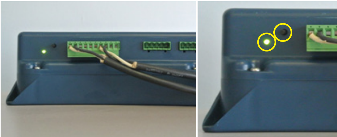
Fig 4: front view of GoRave AR enclosure showing Receive/Send button, LED indicator (highlighted by yellow circle on right) as well as wired speaker outputs and analog audio input.
