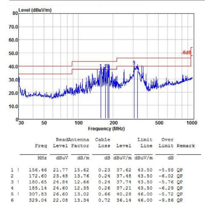
Remark: Absolute Level = Reading Level + Factor, Margin = Absolute Level – Limit Factor = Ant. Factor + Cable Loss
