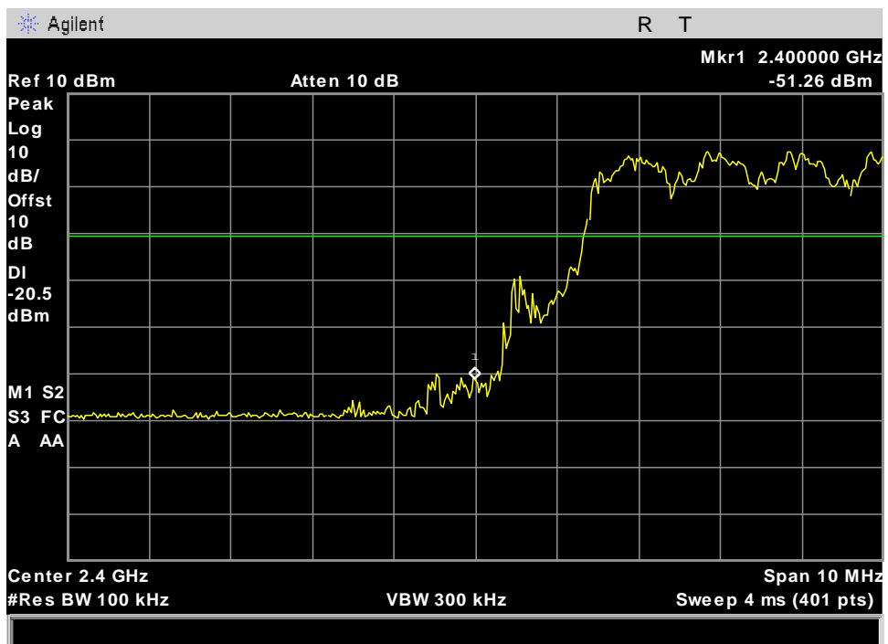
Figure 117: RF Conducted Spurious Emissions Requirements and Band Edge, 100k spurious_2-DH1 hopping_low band edge
