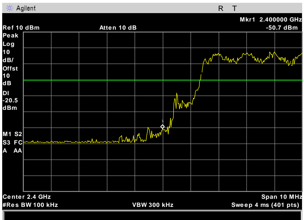
Figure 133: RF Conducted Spurious Emissions Requirements and Band Edge, 100k spurious_3-DH1 hopping_low band edge
