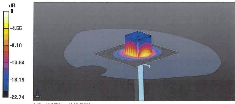
Communication System: UID 0, CW (0); Frequency: 2450 MHz; Duty Cycle: 1:1
