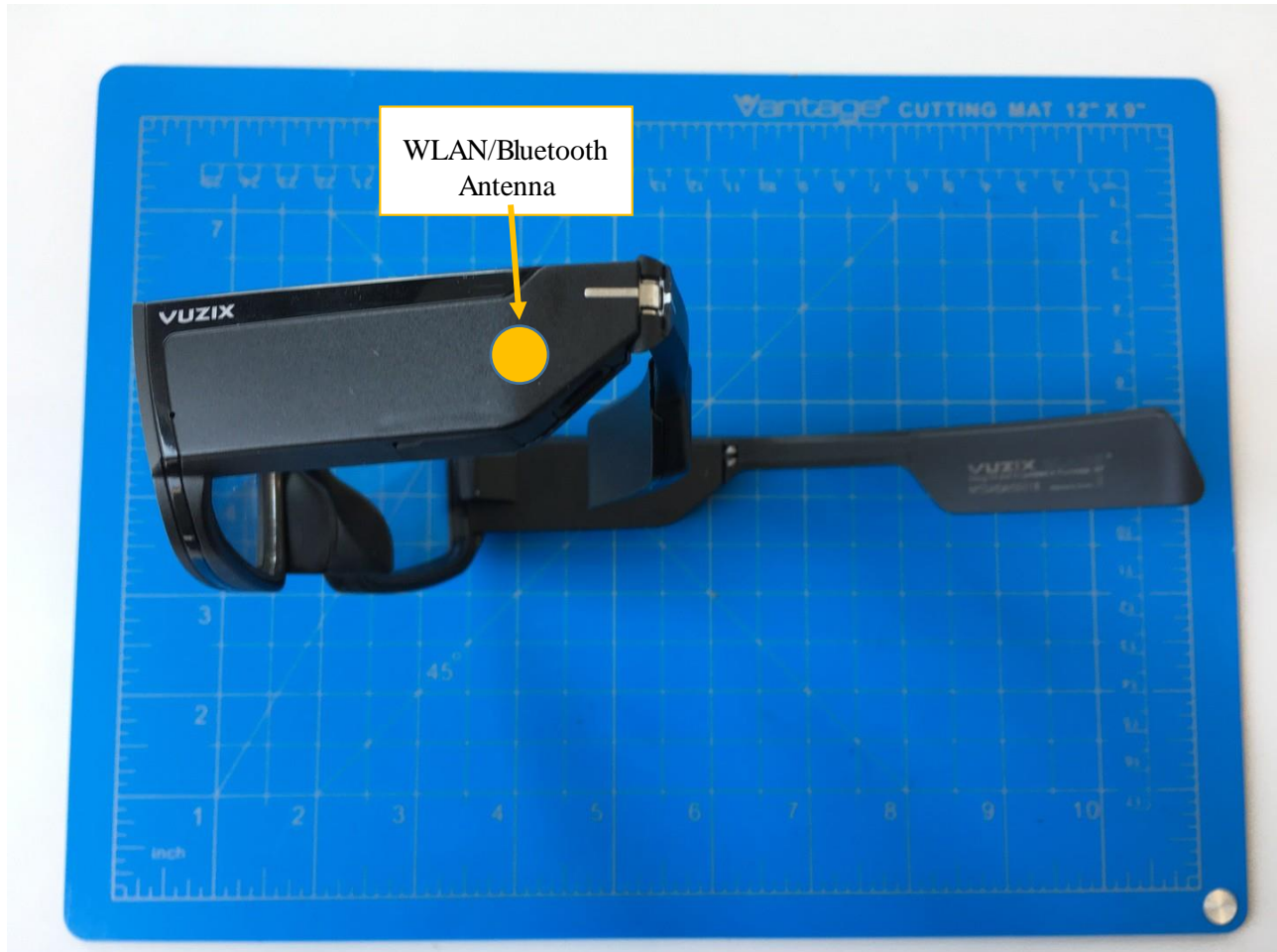
Photo 1: Antenna Location – Normal configuration
