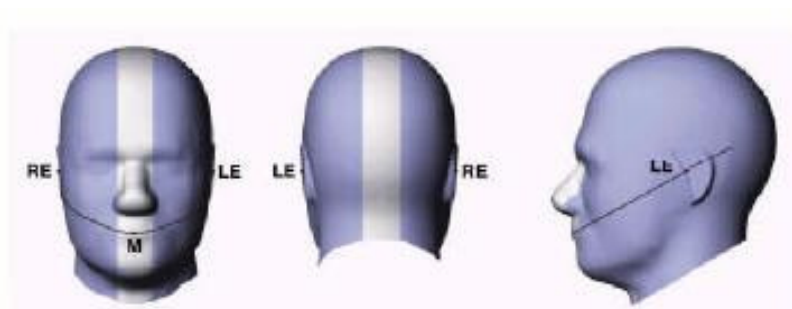
Figure 3: Front, back and side view of SAM Twin Phantom
