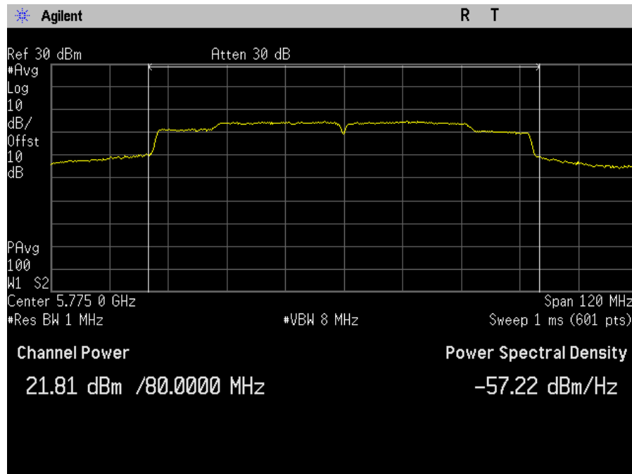
Plot 42. Maximum Conducted Output Power, SISO, Bandwidth 80M, Ch. 5775M, ac mode, port b
