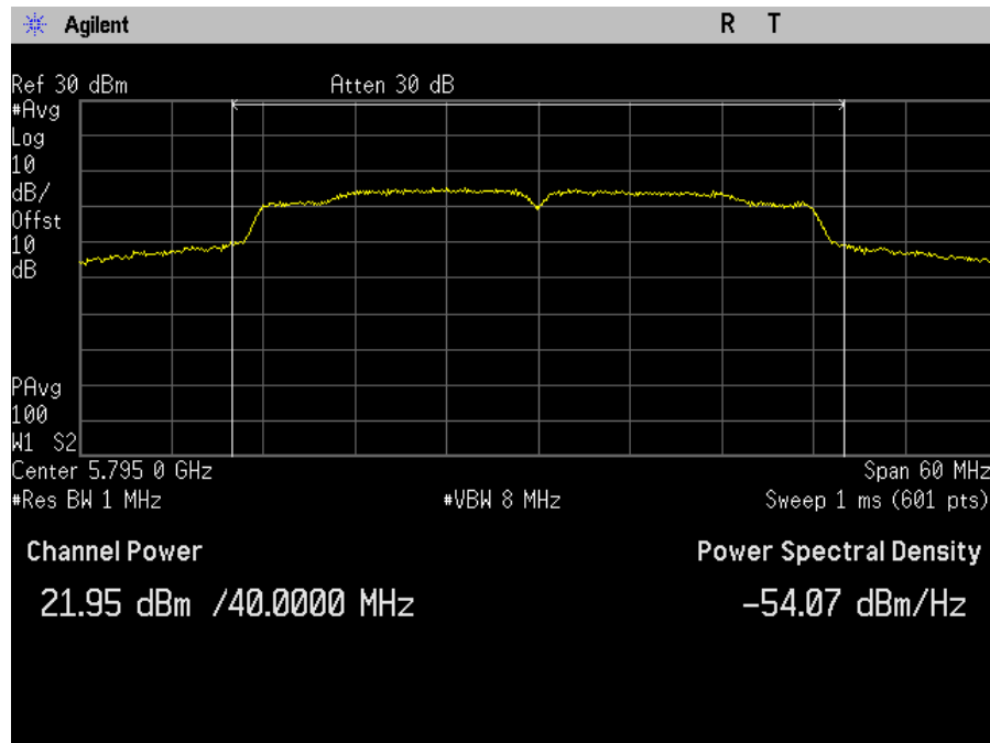
Plot 66. Maximum Conducted Output Power, MIMO, Bandwidth 40M, Ch. 5795M, ac mode, port b
