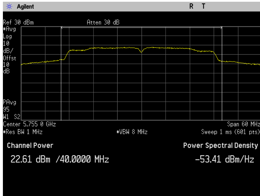
Plot 36. Maximum Conducted Output Power, SISO, Bandwidth 40M, Ch. 5755M, n mode, port b
