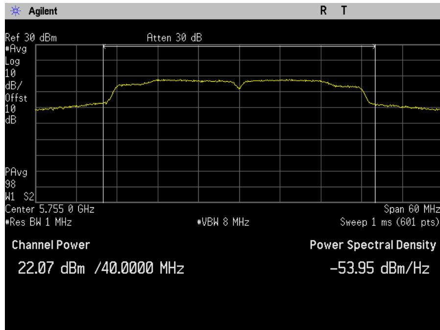
Plot 64. Maximum Conducted Output Power, MIMO, Bandwidth 40M, Ch. 5755M, n mode, port b
