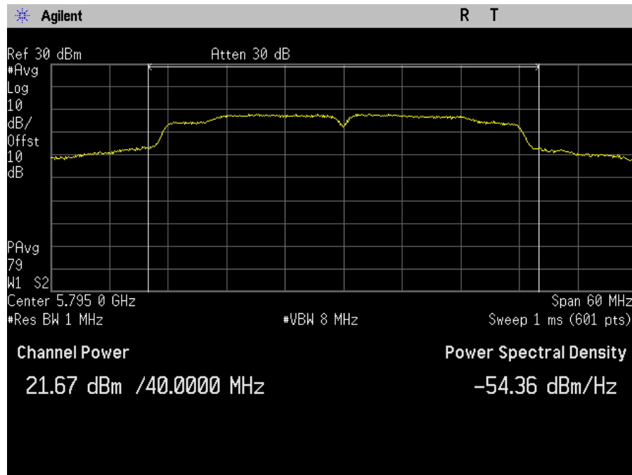
Plot 68. Maximum Conducted Output Power, MIMO, Bandwidth 40M, Ch. 5795M, n mode, port b
