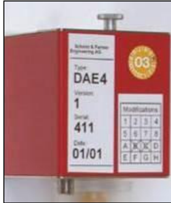
Figure 8: Data acquisition electronics
