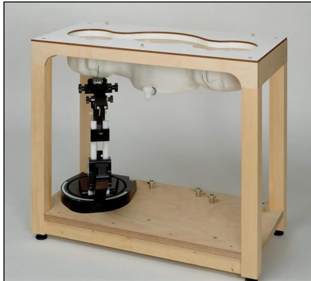
Figure 12: Specific anthropomorphic mannequin twin phantom
