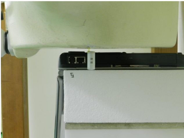
Vertical Front, Test Separation 5 mm
