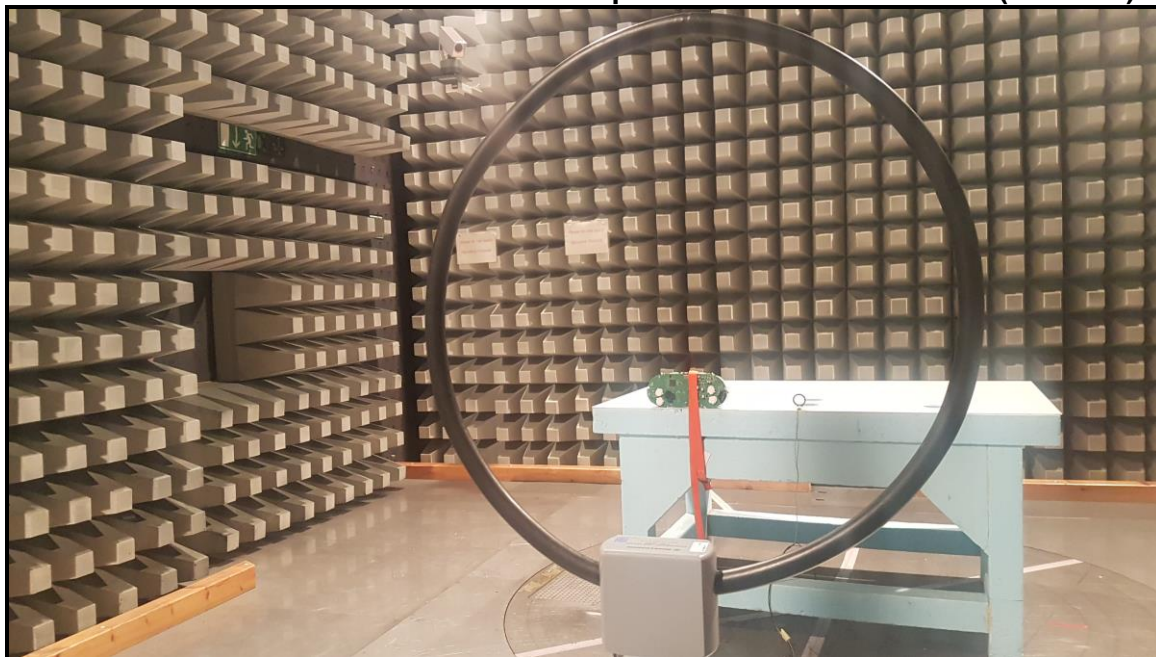
Photo 4: Transmitter H-field & Radiated Spurious Domain Emissions (<30 MHz)
