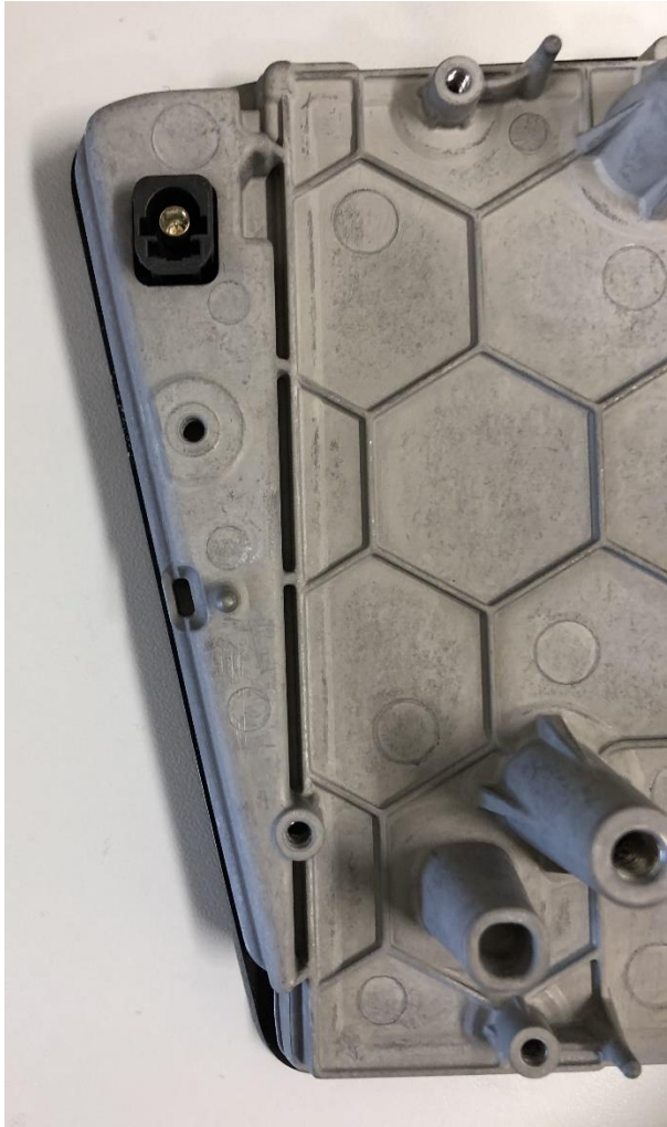
Driver display disassembled backside visible , antenna placed in cavity to the left
