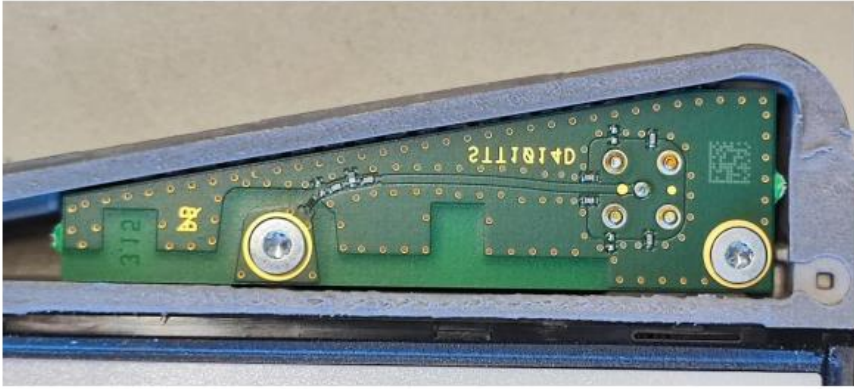
PCB antenna, Right picture antenna in the cavity, direction towards cab
