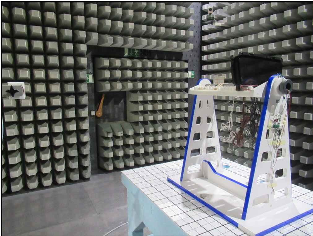
Photo 8 Radiated Test Setup above 18 GHz
