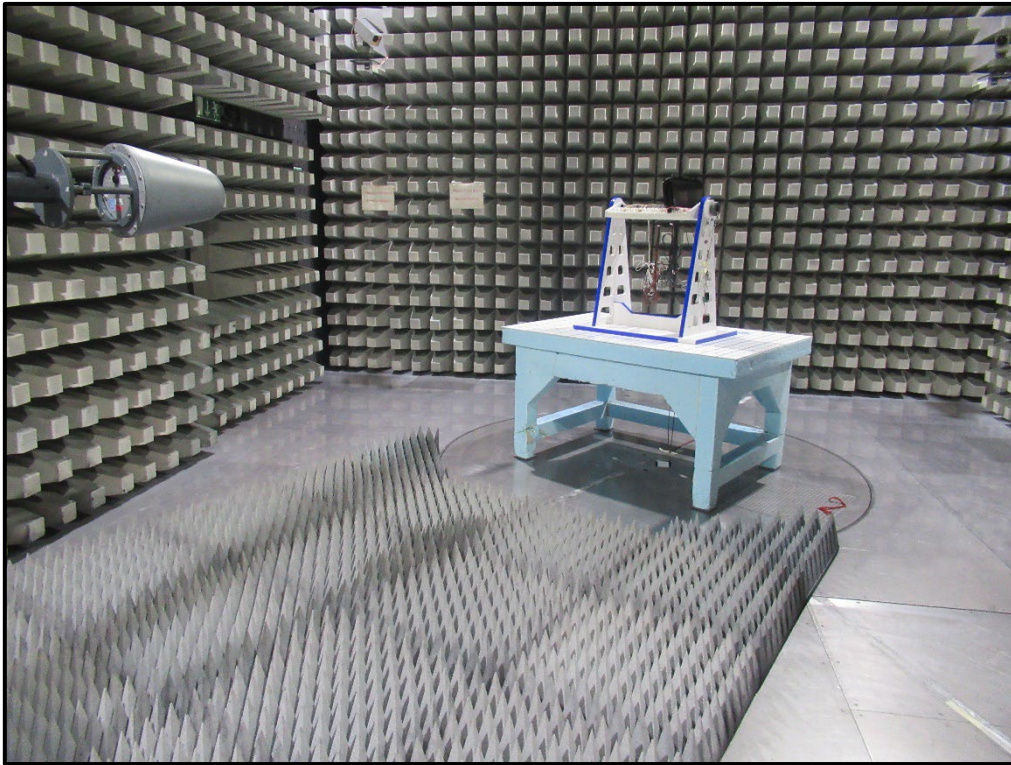
Photo 5 Radiated Test Setup from 1 GHz to 18 GHz
