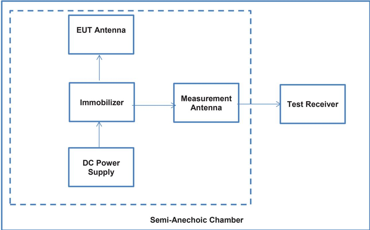
**Transmitter Radiated Spurious Emission test setup (Measurement above 30 MHz)**
