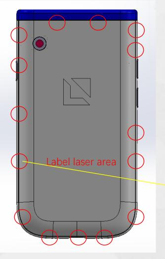
BG1000 back cover which the label laser area is design cannot be openedA. The design has 15 location having snaps design as below. If it opened, it will need to pry it open by using a tools. It will also damage the cover and the housing.
