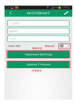
3.2. In the Advanced settings we can set the camera's advanced features: reset the password, motion detection (arming switch, linkage SD card capture, video), scheduled recording, time settings, reboot the device.
