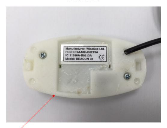
Label with FCC ID:2AA8H-B0213A is located at the rear side panel of the device. The statement according to FCC part 15 §15.19(a)(3) is placed in User's Guide, page 4 (Application exhibit User\_manual\_24511).
