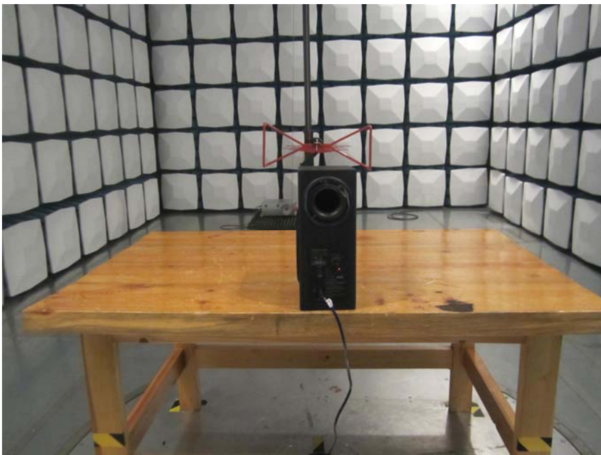
Radiated Emission - Rear View (Below 1GHz)
