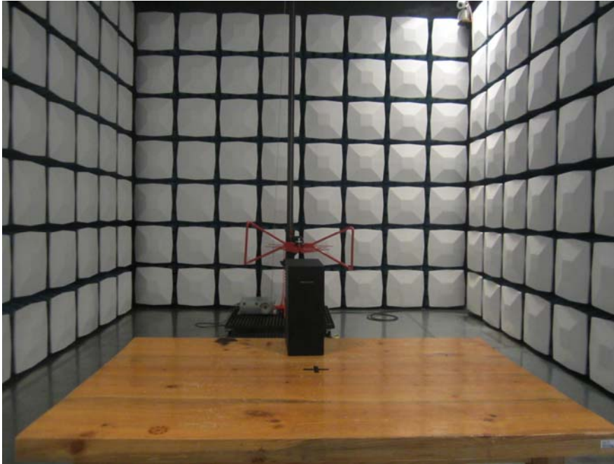
Radiated Emission -Front View (Below 1GHz)
