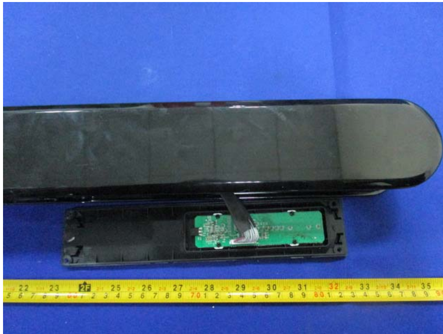
EUT-Other PCB Uncover View
