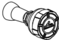
4.Finish, then apply soap water on the sensor to see if leaking.
