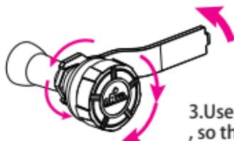
3.Use wrench to fasten the bot counter clock-wise , so the sensor & bolt will lock tightly.
