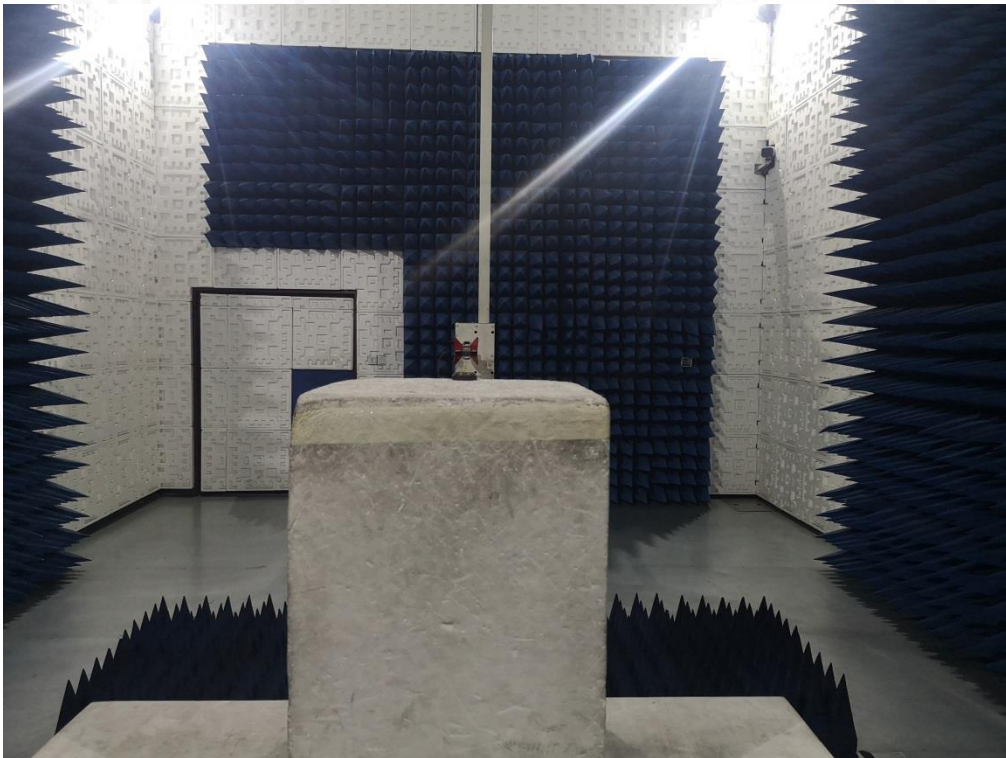
RADIATED EMISSION TEST SETUP ABOVE 1GHZ
