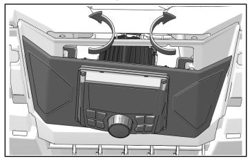
7. Secure PMX head unit to dashboard with four fasteners (10).
