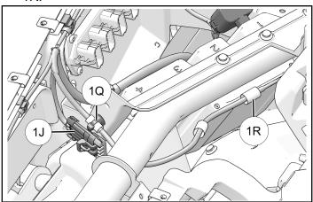
7. Route audio harness to passenger side. Secure to front cab panel with four routing clips 1Q.
