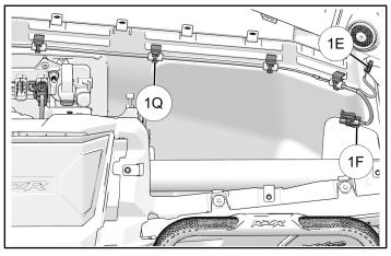
8. Join audio harness connector 1E to tweeter and connector 1F to driver.
