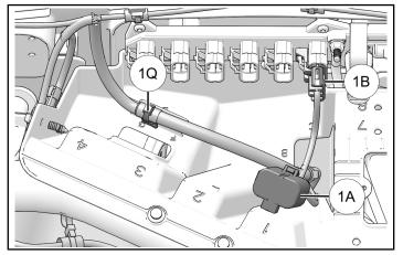
Route amplifier connector 1C and 1D through bottom opening of accessory mounting panel. Secure harness to accessory mounting panel with one routing edge clip 1Q. Join audio harness connectors 1C and 1D to amplifier.
