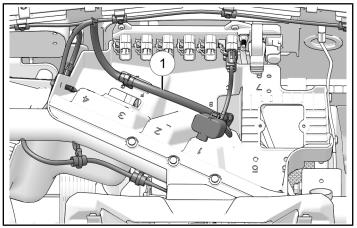
2. Install fuse relay 1A onto accessory mounting panel. Join power connector 1B to Polaris Pulse® bar. Secure harness to accessory mounting panel with one routing edge clip 1Q.
