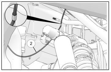
2. Pass harness (2) through grommet in firewall.
