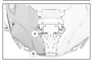
2. Reinstall right-hand hood panel with three hood fasteners (A).
