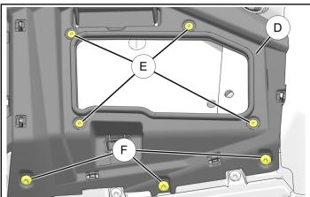
3. Tilt steering wheel down. Remove and retain four screws (£) from dashboard top (D).
