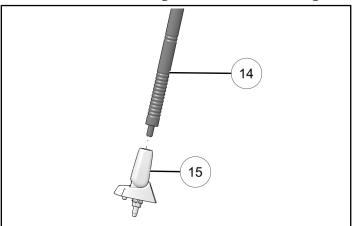
2. Seat antenna mount (§) in hood. Antenna mount will snap into place when fully seated.
