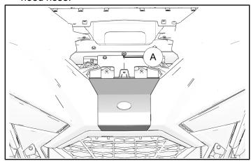
2. Remove and retain three front fender fasteners (A).
