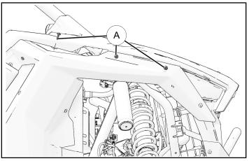
3. Remove and retain one hood fastener (A) and one push-pin rivet (B).
