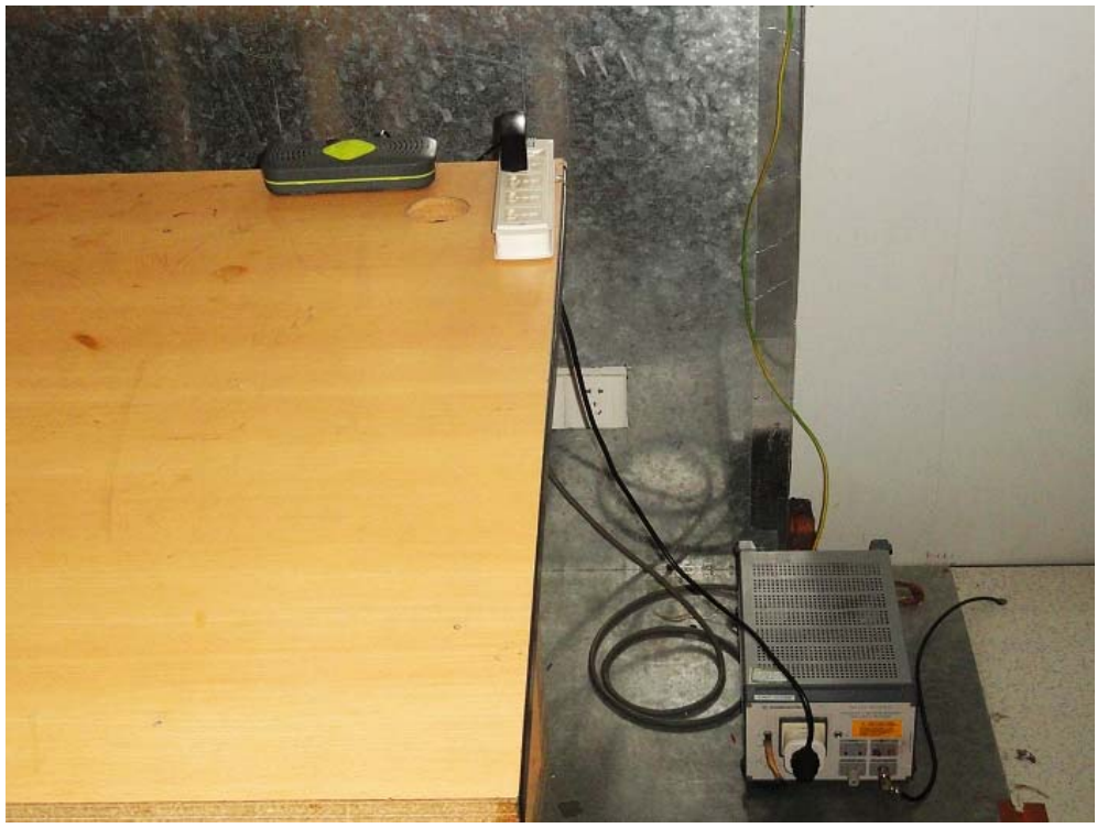
Conducted Emission Test Setup:
