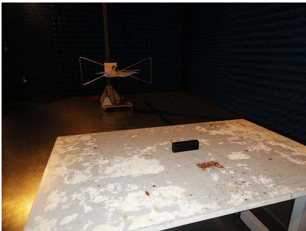
Radiated Emission Test Setup:
