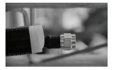
Connect the cable connector with the antenna. Tighten the connection properly with a torque wrench to ensure the correct internal seals and surface contacts are made.
