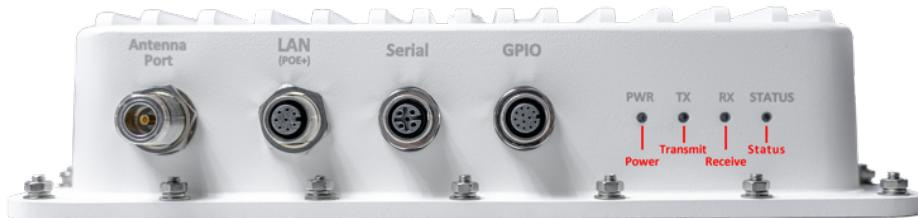
**FIGURE 1 - Connector and LED indicators**
