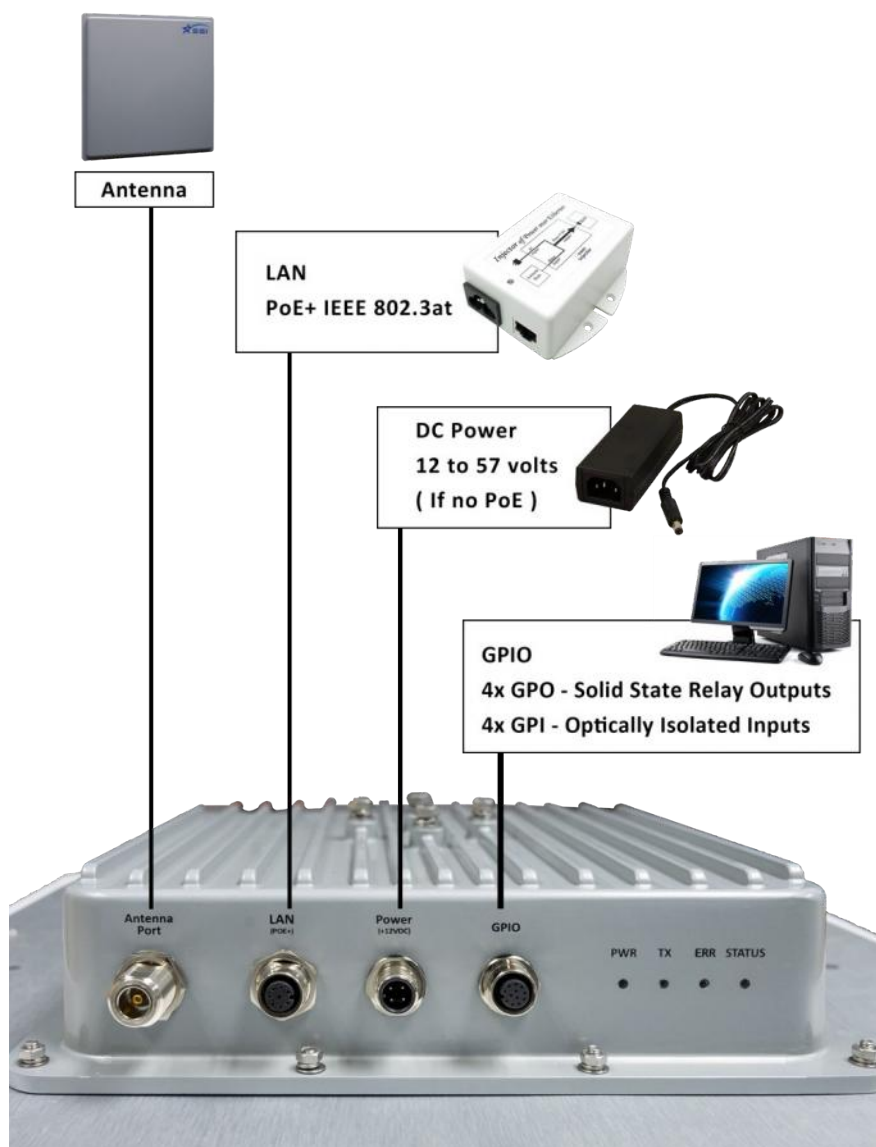
Figure 3. SOLARIA connection diagram
