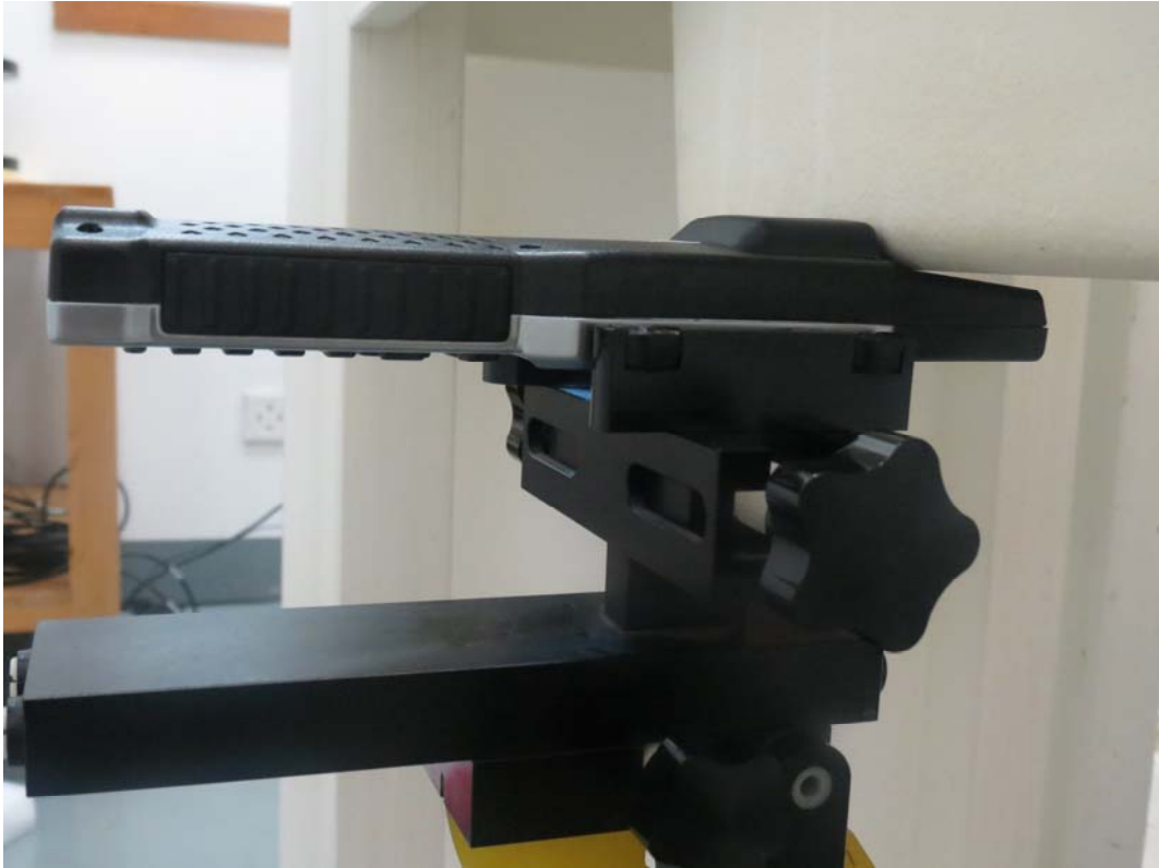
Picture 8: Back Side, the distance from EUT antenna to the bottom of the Phantom is 0mm
