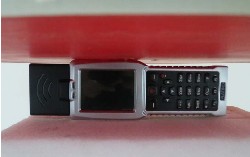
Picture 6: Right Edge, the distance from EUT to the bottom of the Phantom is 0mm
