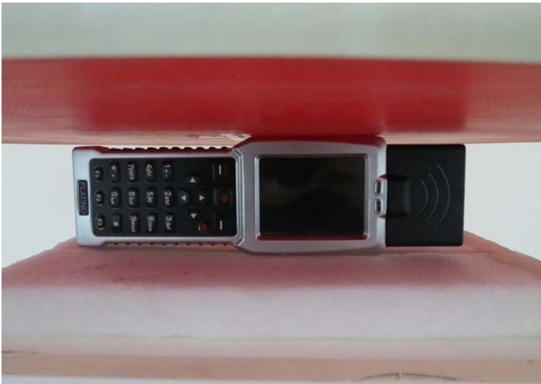
Picture 5: Left Edge, the distance from EUT to the bottom of the Phantom is 0mm
