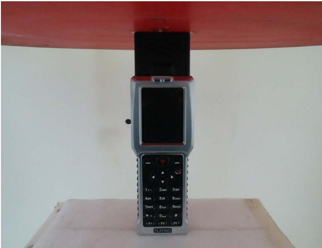
Picture 7: Top Edge, the distance from EUT to the bottom of the Phantom is 0mm
