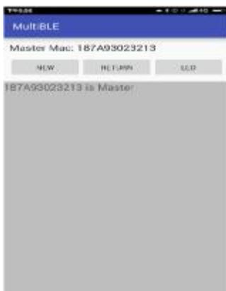
5. Press the "LED" button, the smart terminal will send the command to the devices, the LED will flash after receive the command from smart terminal.
