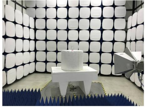
1.2 Radiated Spurious Emissions Test Setup
