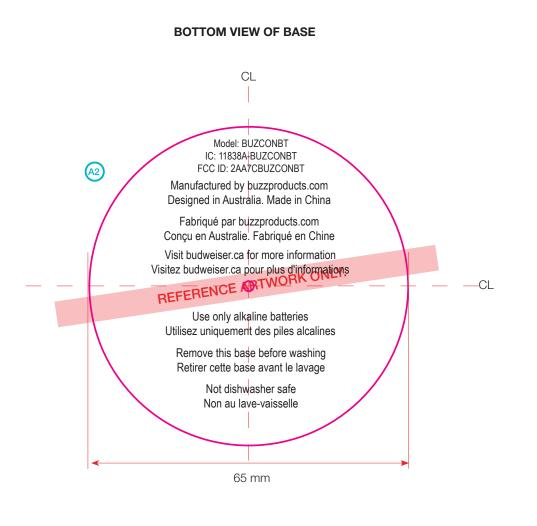
Legal information size: 65mm max type: embossed depth: 0.1mm position: centered on base artwork: LAB012257\_BT\_Base Mould\_ A3.ai
