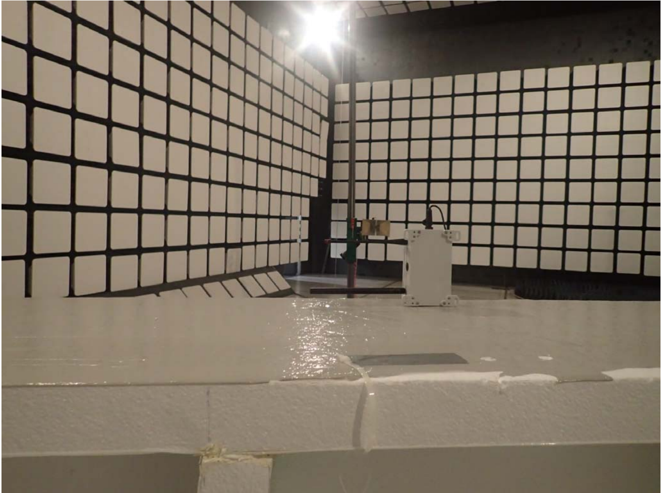
Radiated Emissions at 3m Distance EUT Orientation: Orthogonal Position 3
