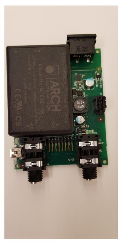
The AC-DC Module ARCHCORP MTC15-30S is filled with potting compound from the manufacturer due to safety reason and can't be opened and photographed inside.
