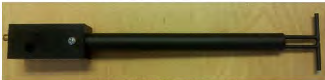
Figure 1 – MVG COMOSAR Validation Dipole
