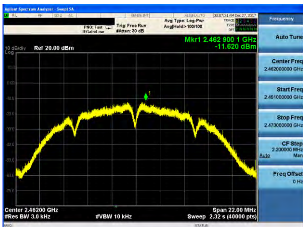
(802.11b) PSD plot on channel 11
