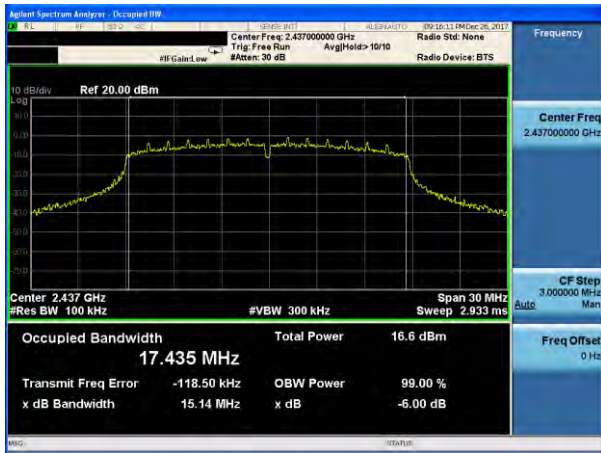
(802.11n20) 6dB Bandwidth plot on channel 11
