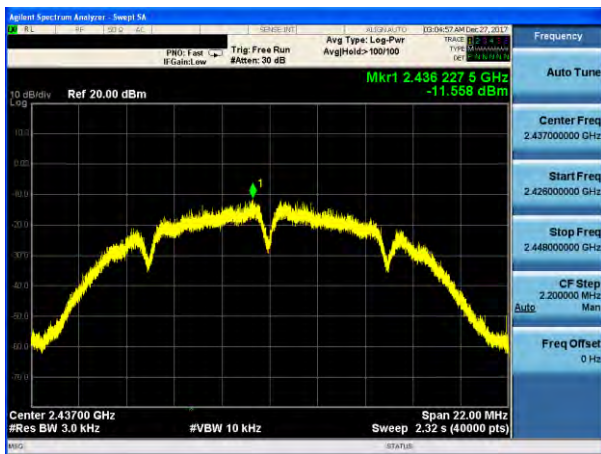
(802.11b) PSD plot on channel 6
