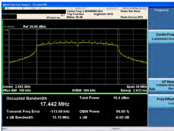
(802.11n20) 6dB Bandwidth plot on channel 11
