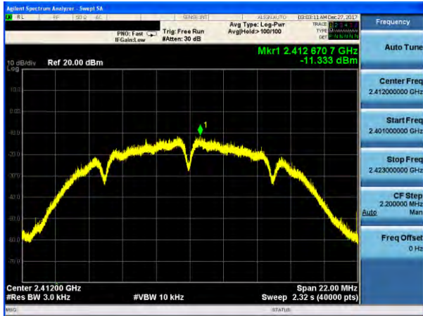
(802.11b) PSD plot on channel 6
