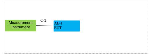
Note: 1. The temporary antenna connector is soldered on the PCB board in order to perform conducted tests and this temporary antenna connector is listed in the equipment list.
