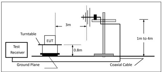
(c) For radiated emissions above 1000MHz
