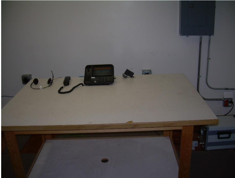
Photograph 1: Front View Conducted Emissions Worst-Case Configuration
