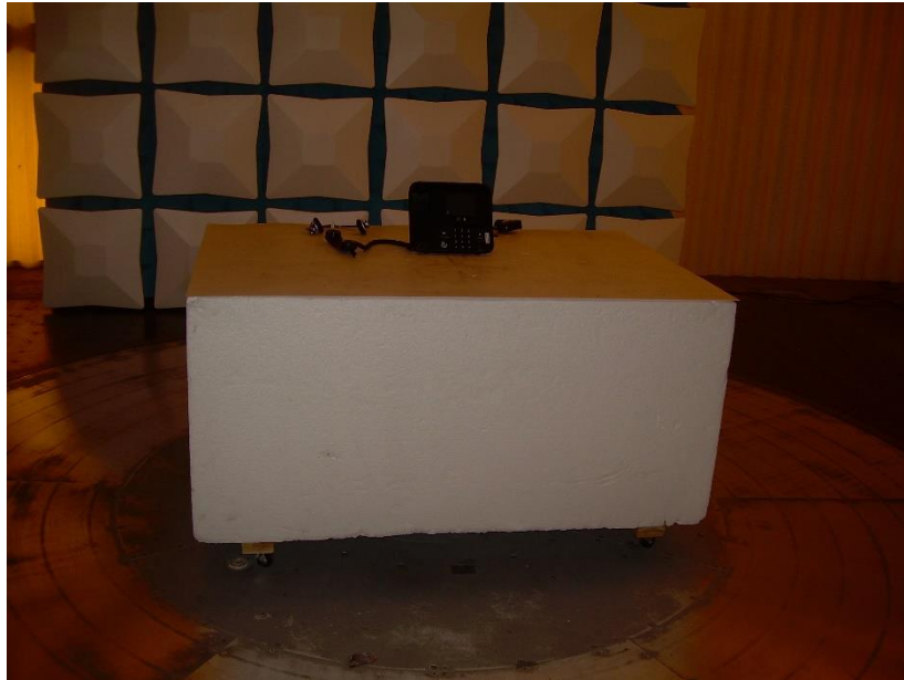
Photograph 3 – Front View Conducted Emissions Worst-Case Configuration – Below 1000 MHz
