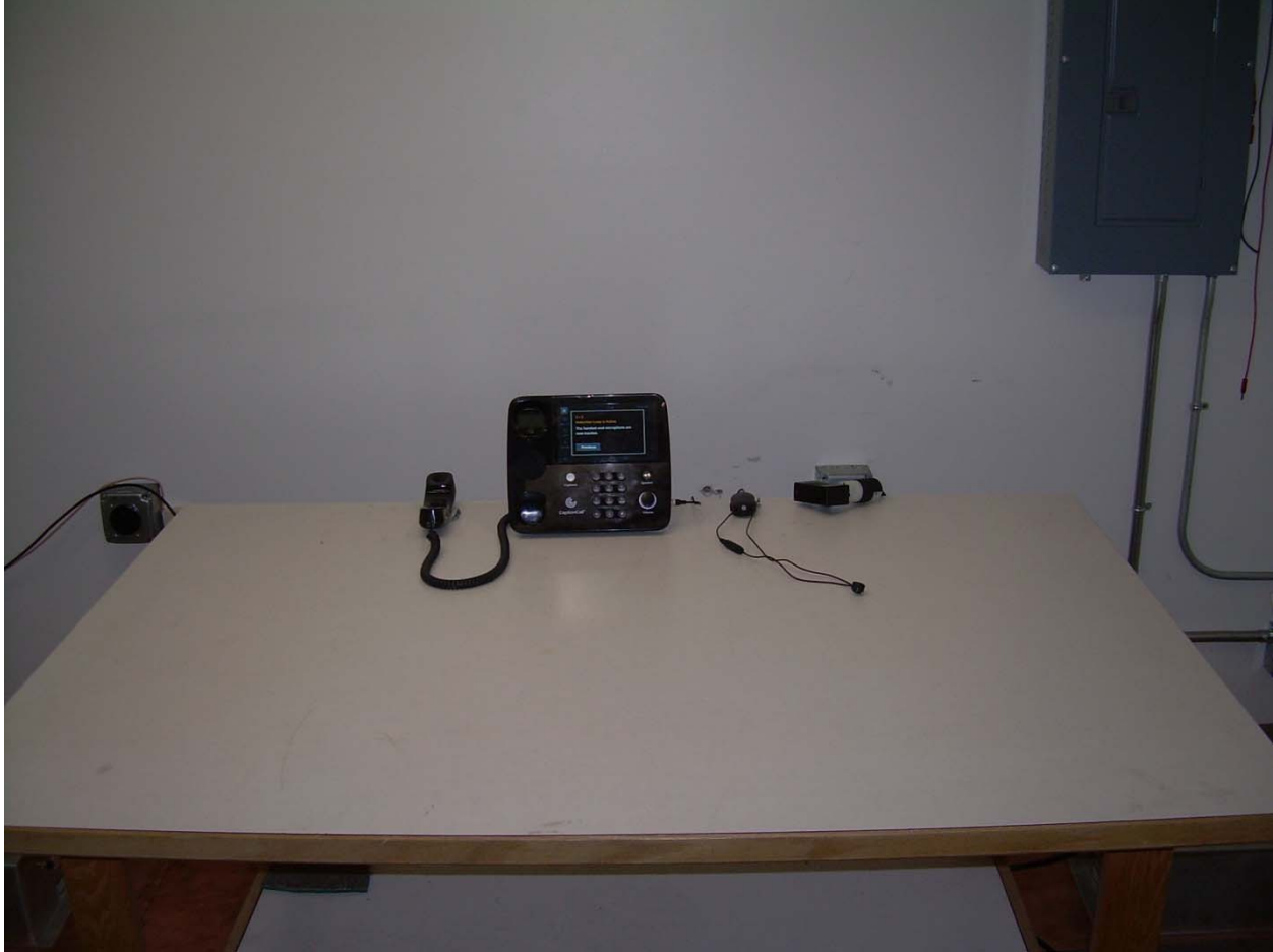
Photograph 3 – Front View Conducted Disturbance Worst Case Configuration
