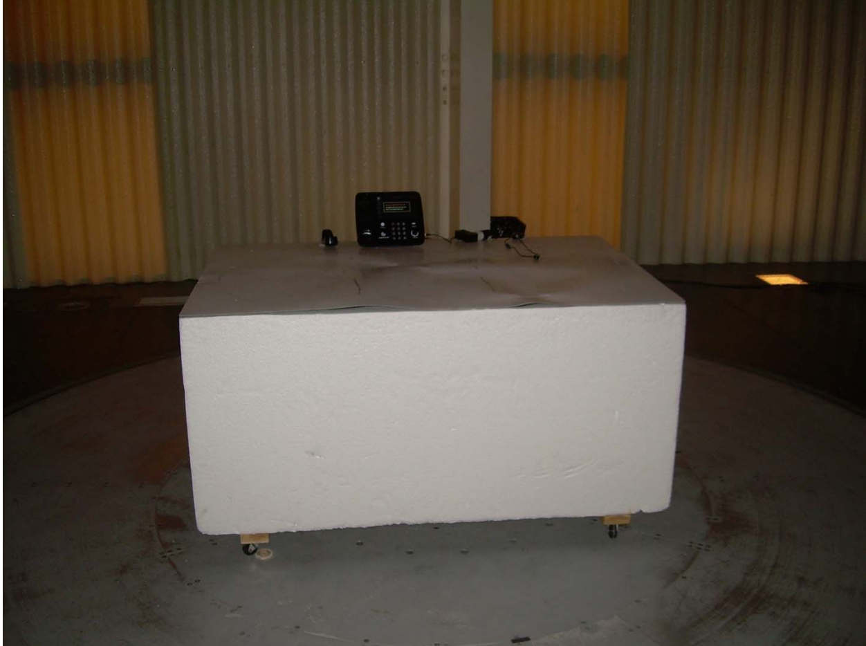
Photograph 1 – Front View Radiated Disturbance Worst Case Configuration
