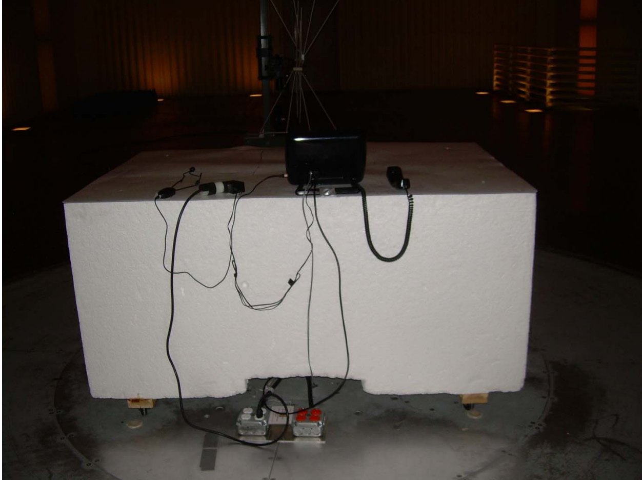
Photograph 2 – Back View Radiated Disturbance Worst Case Configuration
