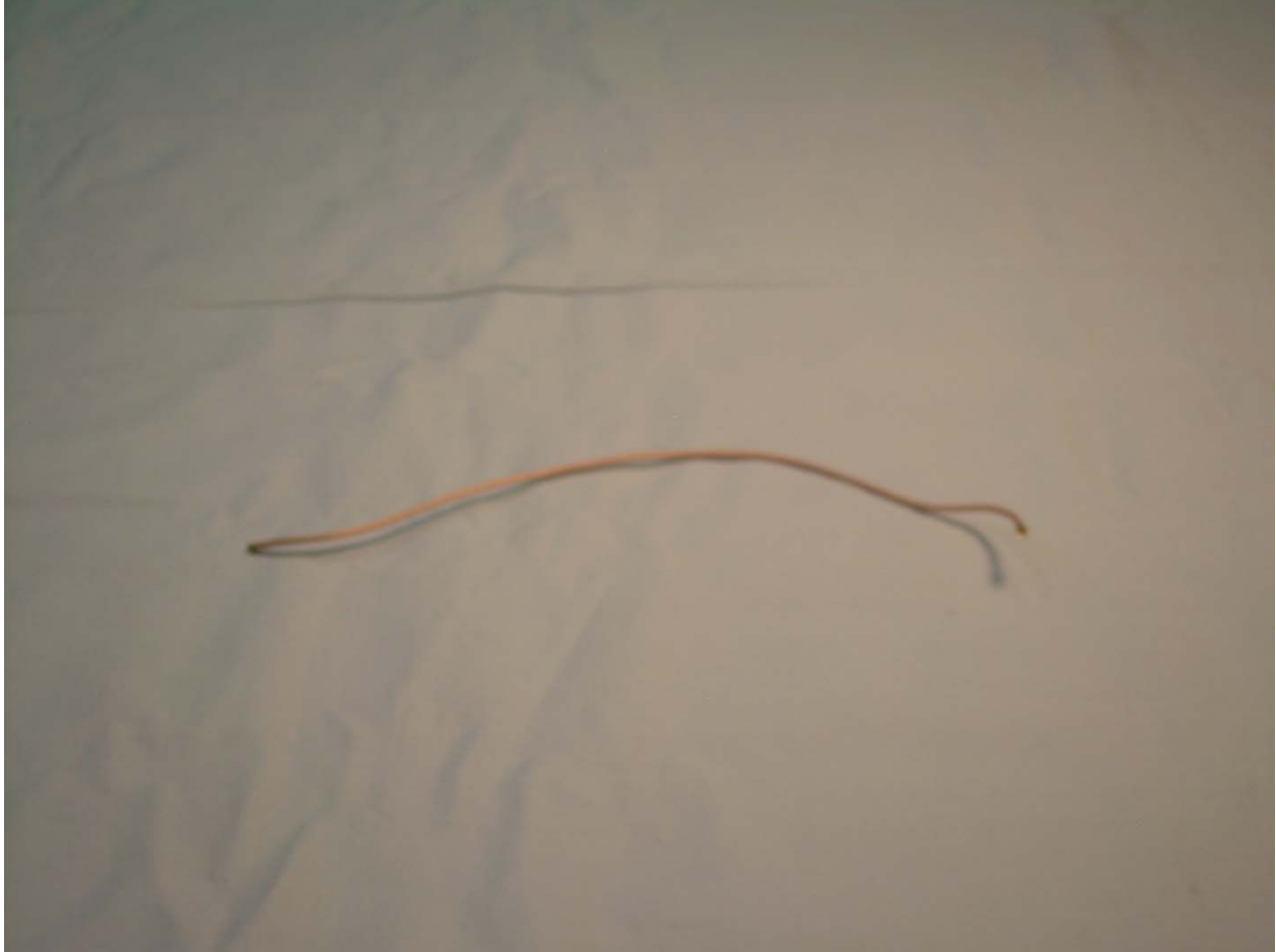
Photograph 15 – View of the Coax Cable that Connects the Main PCB to the Antenna PCB
